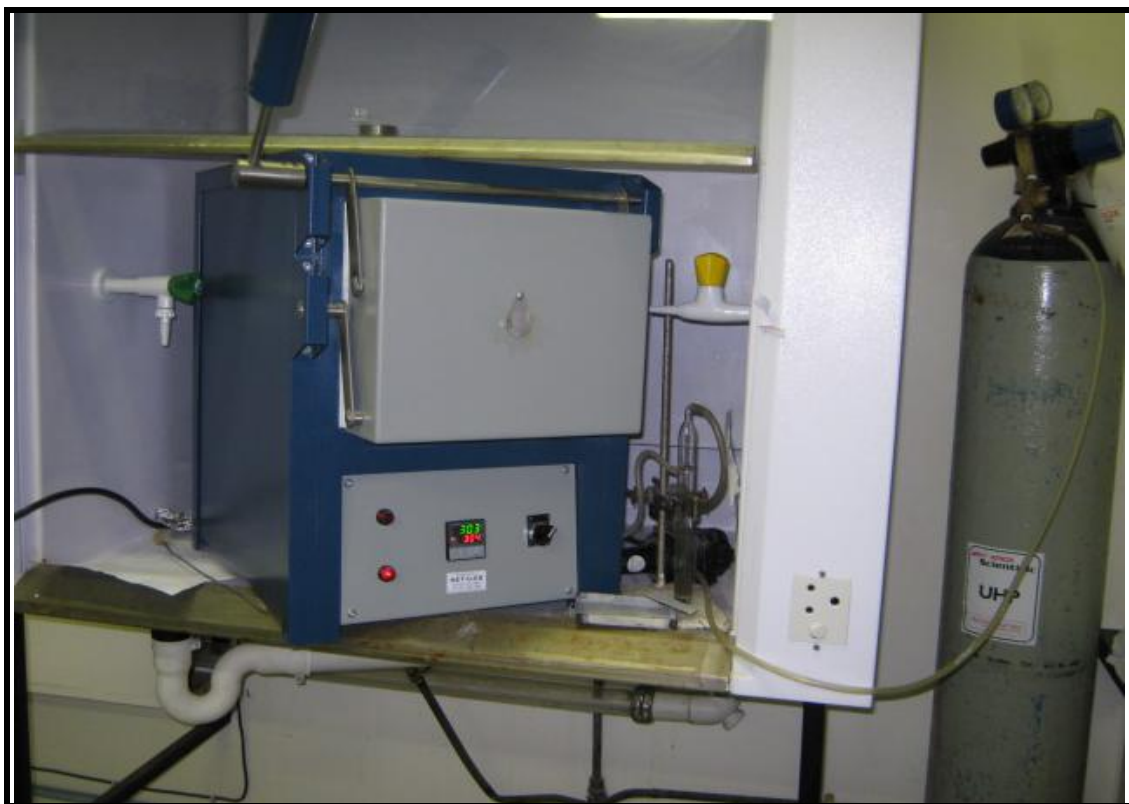
Figure 4.2: A photograph of the furnace used for stabilization, calcination and carbonization.
