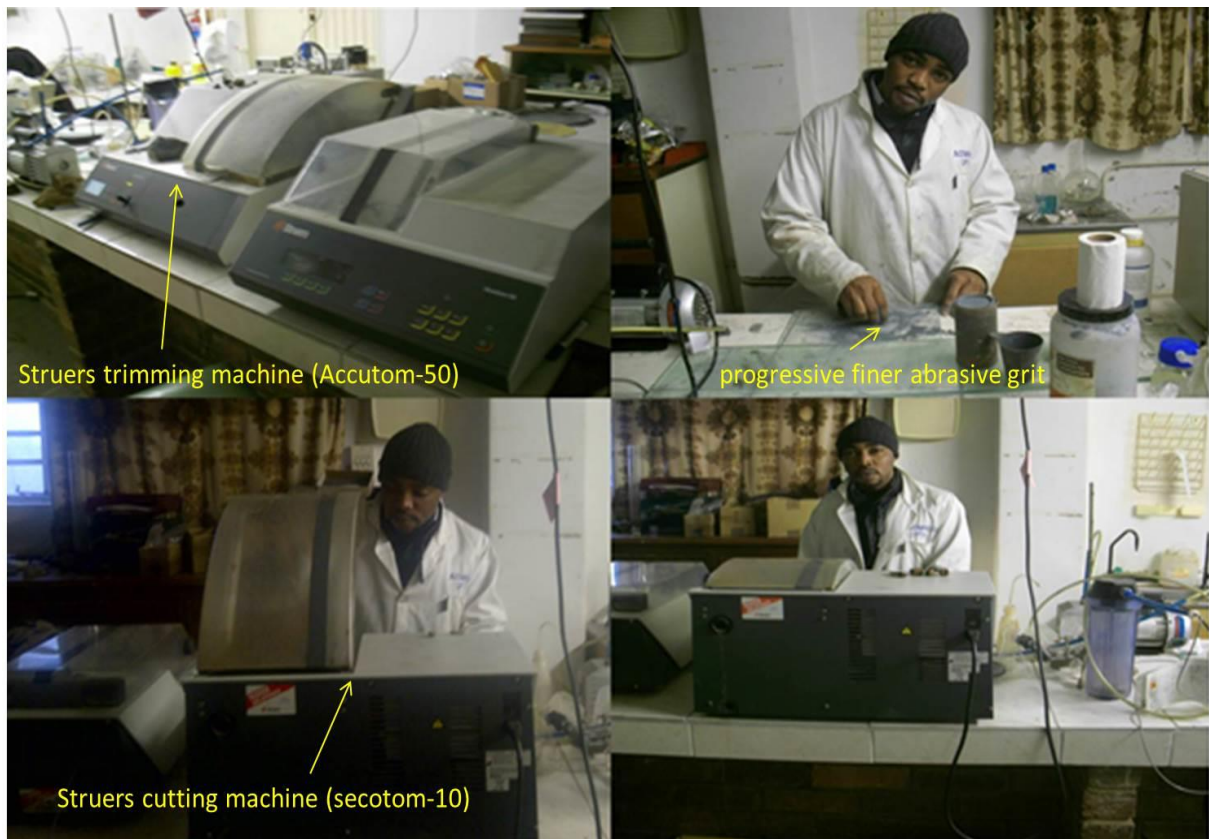
Figure 4.36 Photograph showing thin sections preparation at the Geology department's thin section laboratory, University of Fort Hare, South Africa.
