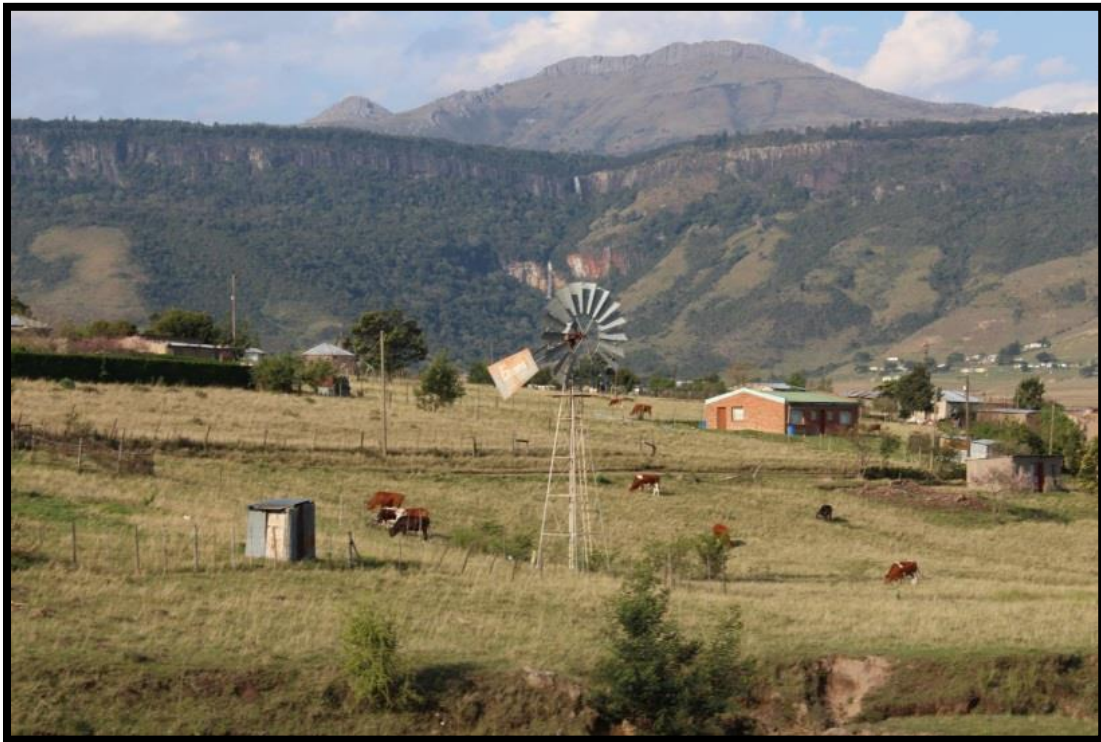
Figure 4.2: Windmill for pumping groundwater to households in Binfield, Eastern Cape, South Africa (2014)
