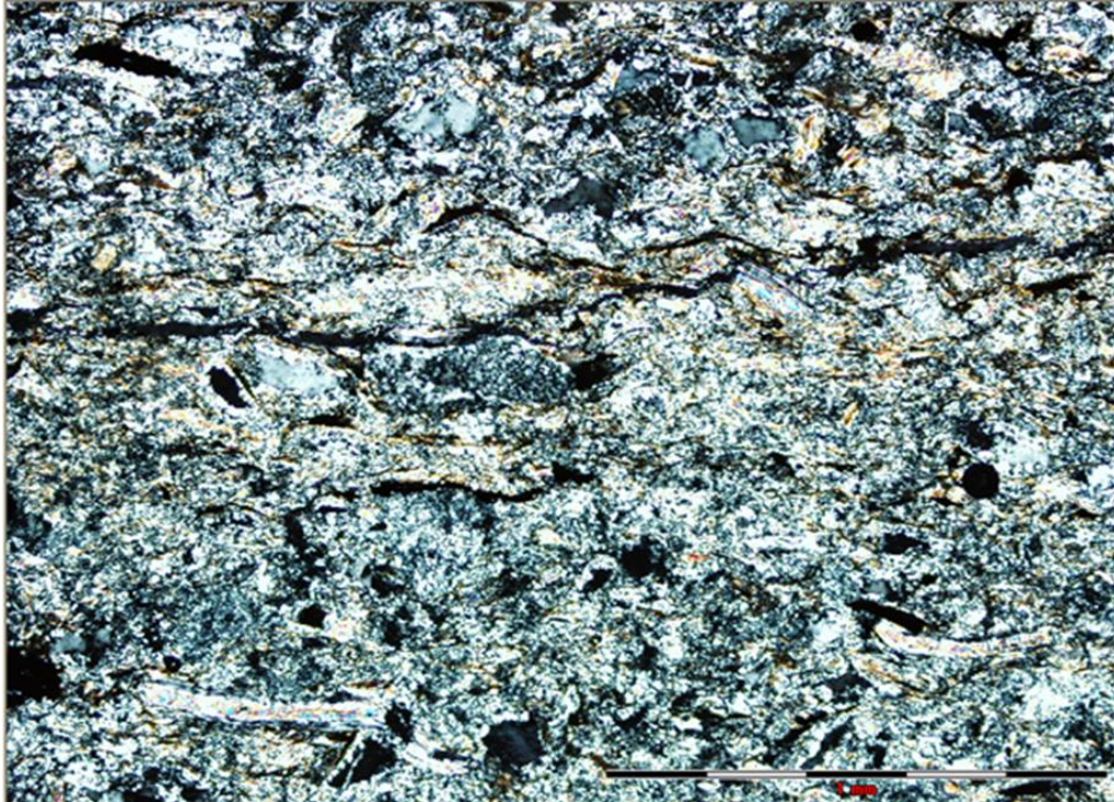
Figure 7.12: Photomicrograph showing mudstone with microfractures and pores in the Margate area.
