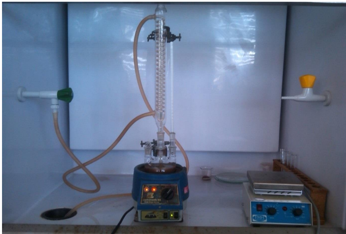
Figure 4.1: PMPSgLig-NaMMT nanocomposite synthesis laboratory reaction setup.
