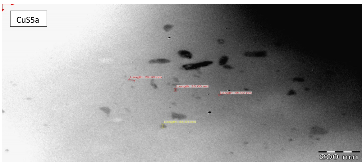
Figure 4.13: TEM images of CuS1a, CuS4a and CuS5a nanoparticles.
