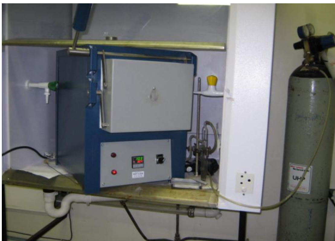
Figure 4.2: Programmable furnace used in the calcination of \text{TiO}_2 and N- \text{TiO}_2
