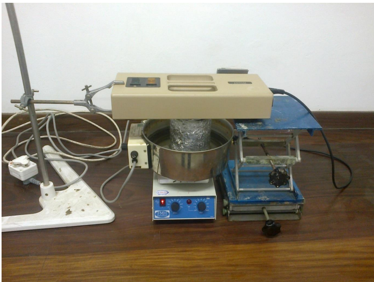
Figure 3.5: Photo-degradation set-up under strict UV light at 25 °C and natural pH
