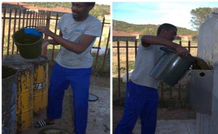
Figure 3. 3. Slurry preparation and feeding of the digester
