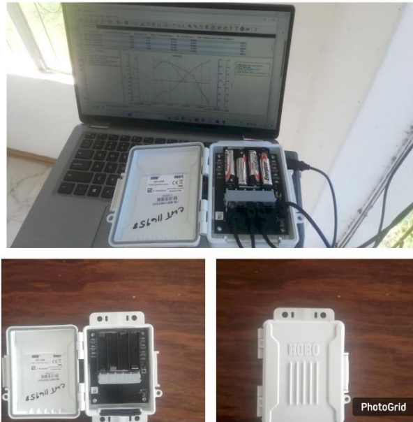
Figure 3. 17. HOBO H21 mini weather station
