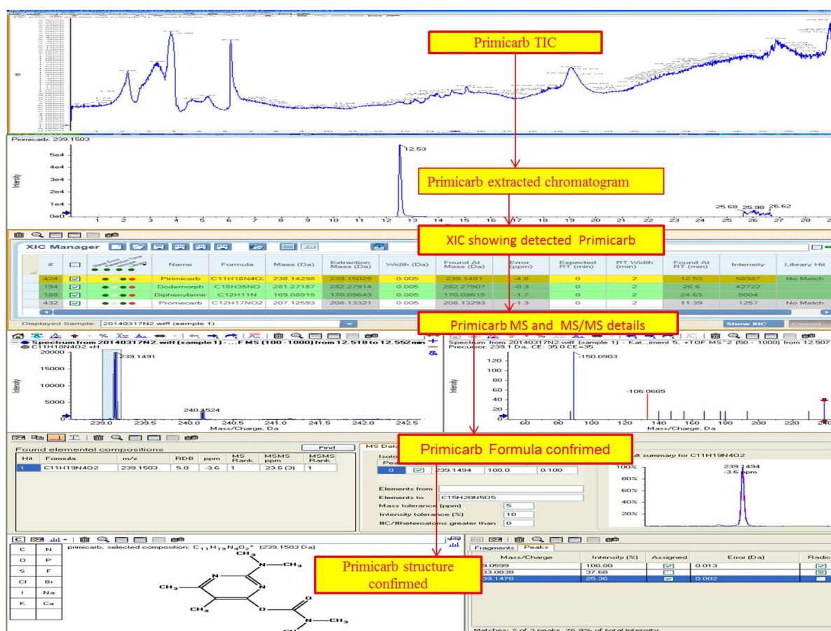
Figure 2-30: Typical example of experimental flow diagram for the identification and confirmation of Primicarb in an Orange sample after running the TIC obtained from an Orange sample against the pesticide library.
