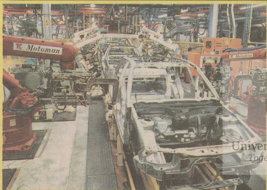
DELTA-NEW OPEL ASTRA AND KADETT ASSEMBLY LINE
