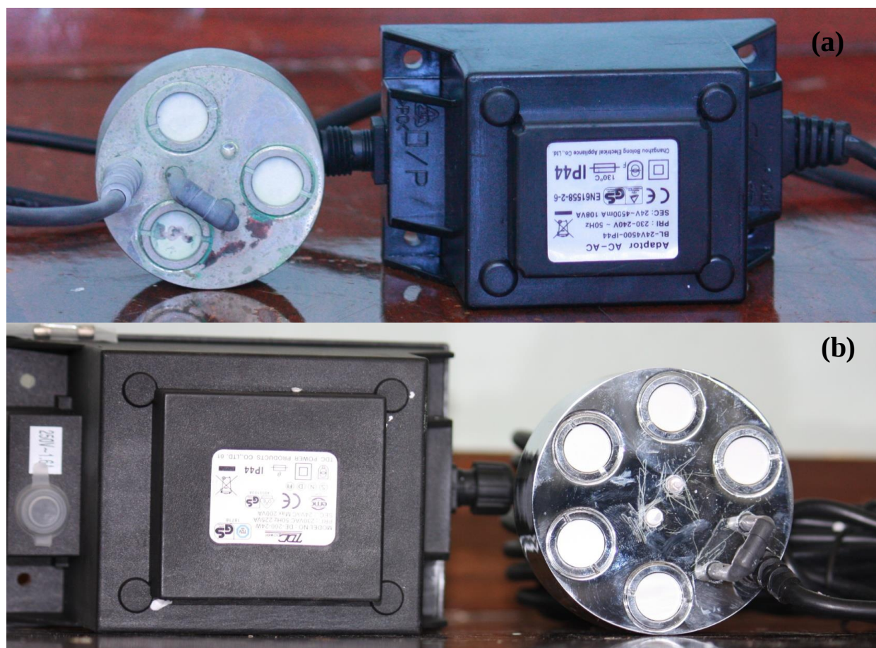
Figure 4.7: Ultrasonic nebulizers employed in the study. (a) Shows the 1.7 MHz ultrasonic nebulizer with power supply unit and (b) shows the 4.8 MHz ultrasonic nebulizer with power supply unit.
