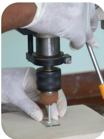
Figure 5.3: Experimental procedure for drilling holes in FTO glass substrate prior to platinum coating, for subsequent electrolyte injection.
