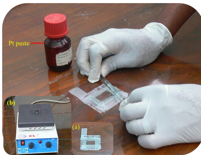
Figure 5.6: Coating of the Pt-catalyst to the photo-cathode. Insert (a) shows the glass substrate fixed with adhesive tape before doctor blading of Pt catalyst onto FTO glass substrate (main picture). Insert (b) Firing of the Pt catalyst on a hot plate
