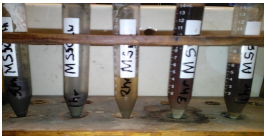
Figure 5.5: Colloidal solutions of Ag-NPs synthesised using 1 g ethanolic extract and 5 ml of 0.1M AgNO 3
