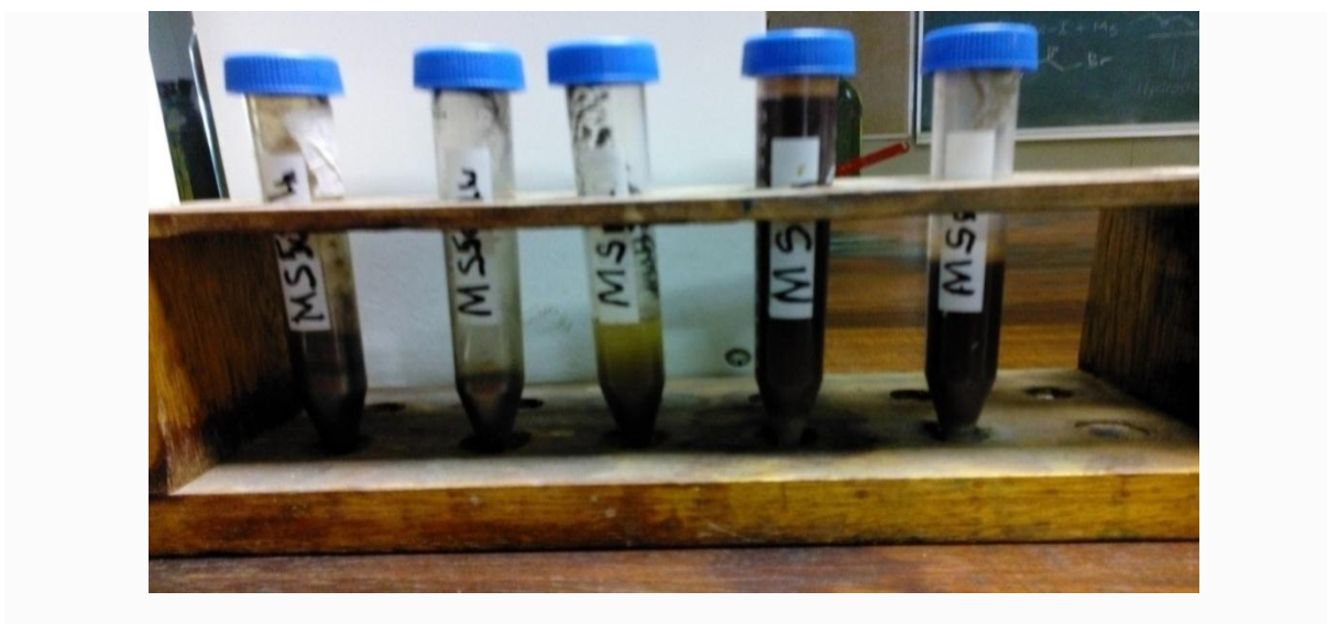
Figure 5.3: Colloidal solutions of Ag-NPs synthesised using 5 ml hydrosol and 5 ml 0.1 MAgNO 3
