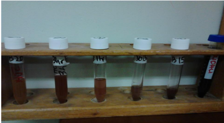
Figure 6.3: Colloidal solutions of Ag-NPs synthesised using ethanolic extract at 60°C at different reaction time.
