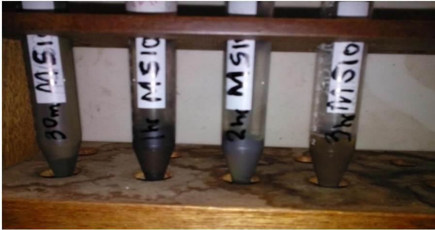
Figure 5.1: Colloidal solutions of Ag-NPs synthesised using 5 g ethanolic extract /1ml, 1M AgNO 3
