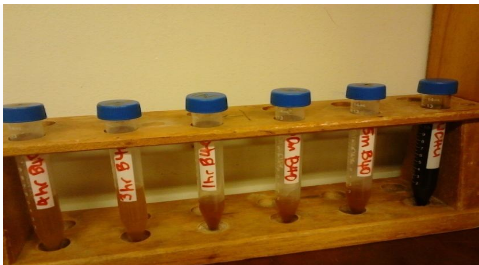
Figure 6.1 Colloidal solutions of Ag-NPs synthesised using ethanolic extract at 40°C at different reaction time.
