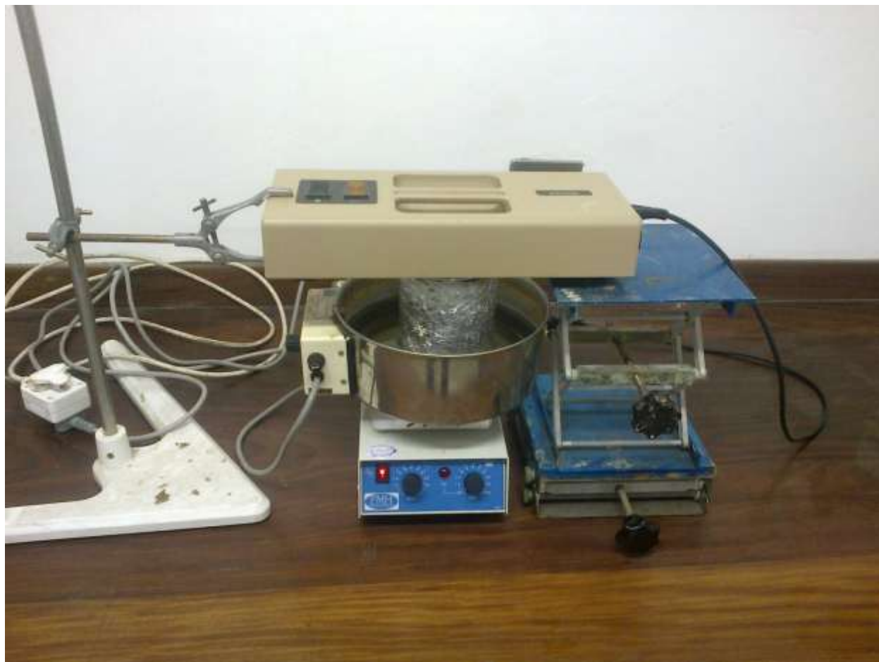
Figure 5.1: Photo-oxidation reactor setup
