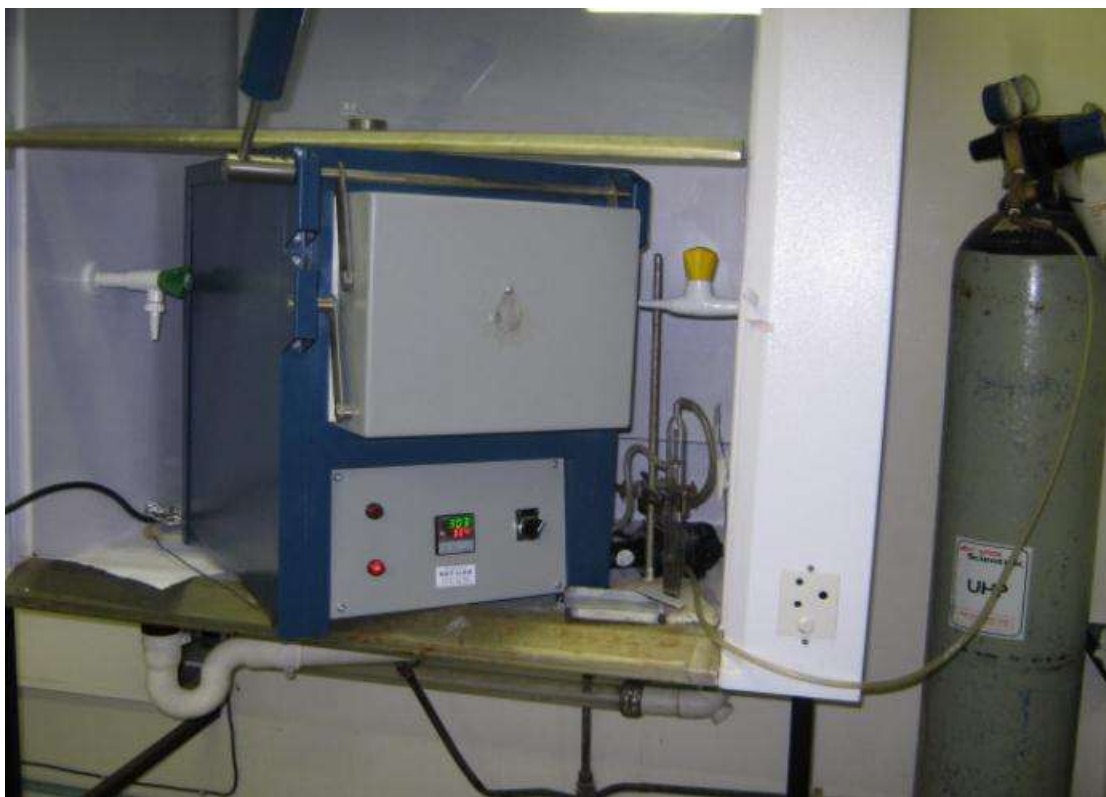
Figure 4.2: Programmable muffle furnace for calcination
