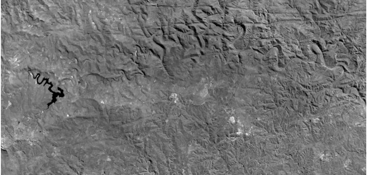
Figure 4- 20: Example of negative weathering of dolerites depicted as lineaments
