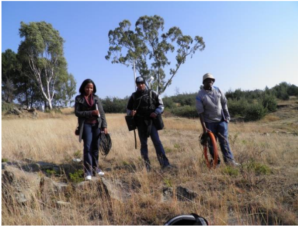
Figure 7- 4: One of the coil (orange circumference) that was used to acquire electro-magnetic data
