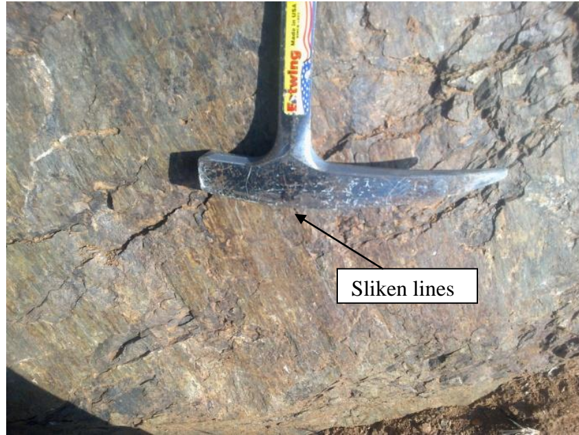
Figure 4- 42: Dip-slip movement indicated by the occurrence of slicken lines on a surface of siltstone
