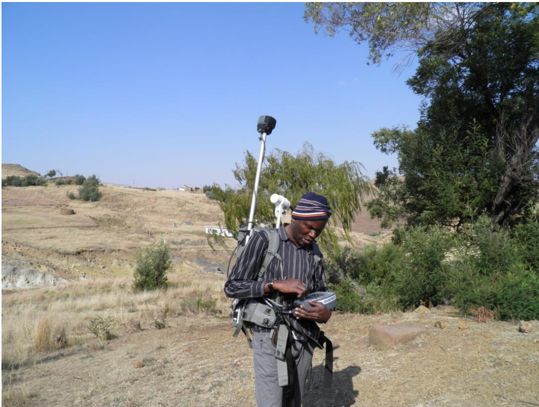
Figure 7- 3: Proton precession magnetometer that was used for data acquisition (Polile Tshisa hot spring)
