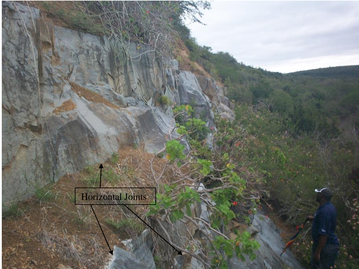
Figure 5- 22: Dolerite sill with horizontal joints infilled with quartz veins.
