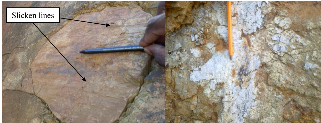
Figure 6- 10: left) Lineation on a quartzite breccias showing horizontal movement; right) dip-slip movement parallel to the pen seen on a coated surface of a reactivated fault.
