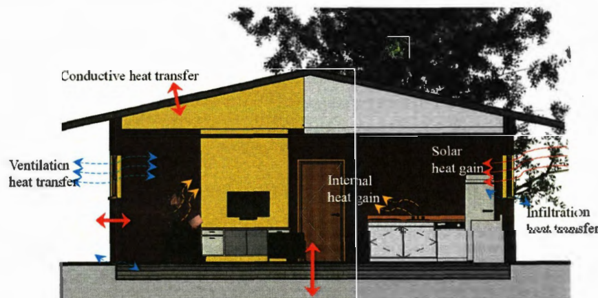
Figure 2.1: Schematic of a building thermal load
