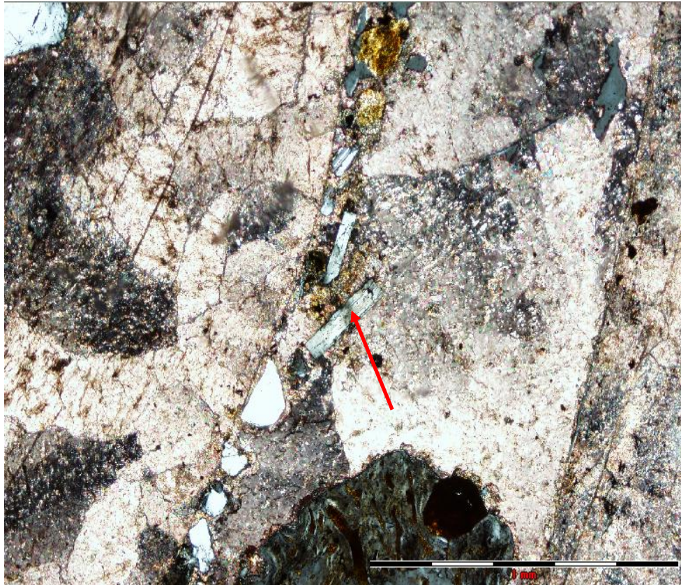
Figure 80: Authigenic feldspar, with cleavage planes (arrow).
