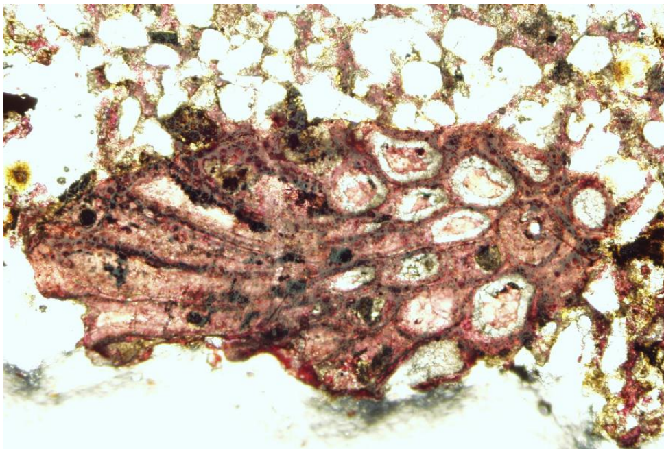
Figure 66: Pore-filling texture in a bioclast.
