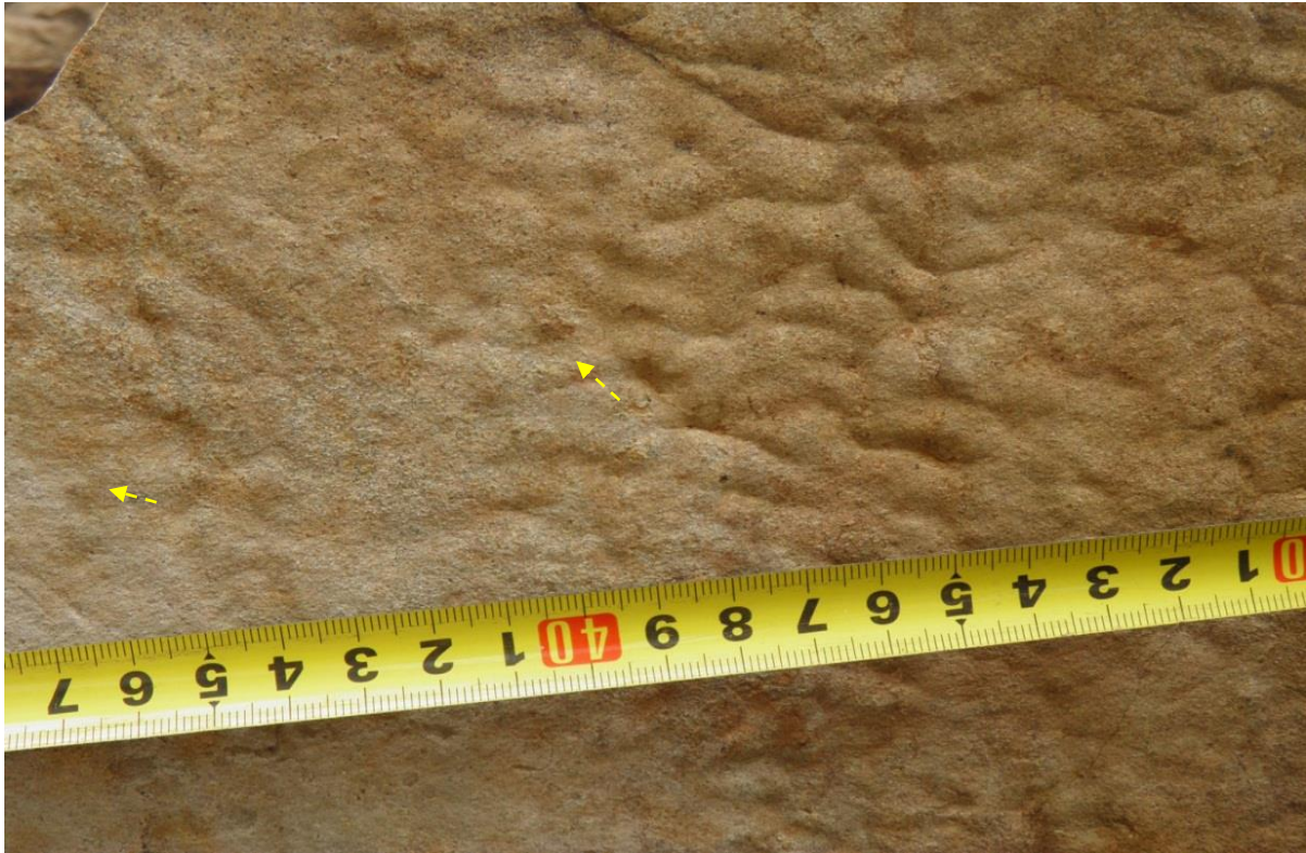
Figure 4.10 Node clasts at the bottom surface of a sandstone rock.
