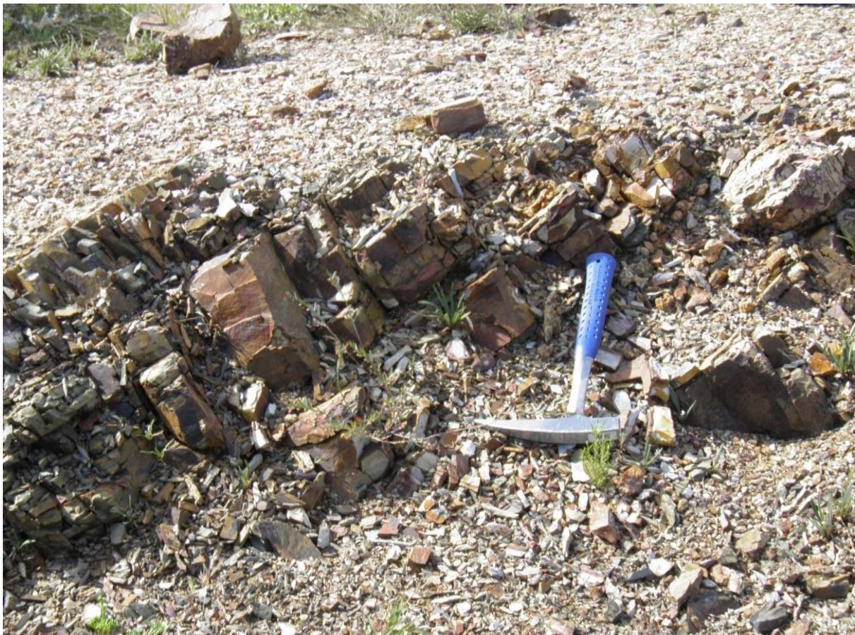
Figure 6.1 Weathered laminated khaki shales, with fine siltstone lenses.
