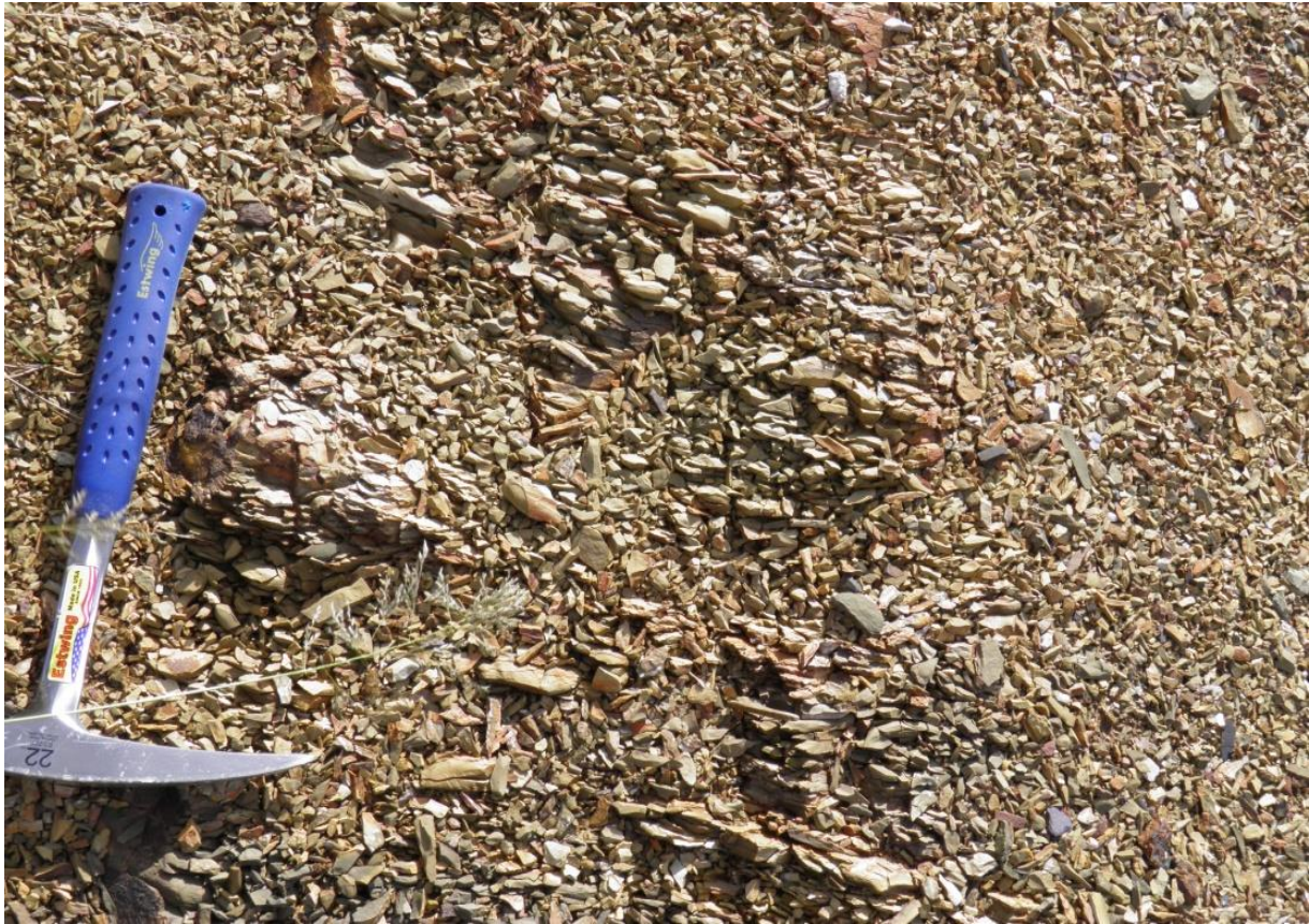
Figure 4.11 The crumbling of shale along lamination planes.
