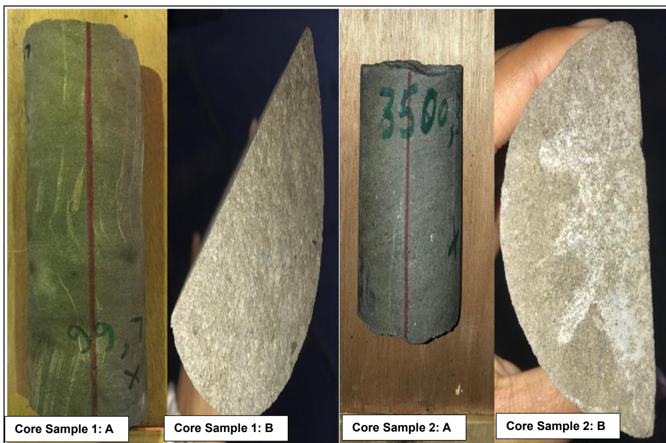
Figure 5.4 Core samples for E-G2. Core Sample 1A and B: 3499.47 m. Core Sample 2A and B: 3500.30 m.
