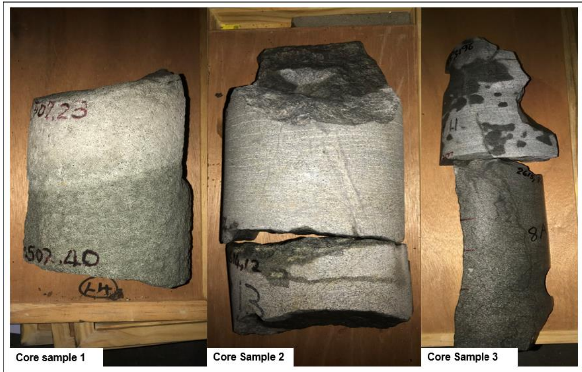
Figure 5.3 Core samples for E-AQ1. Core Sample 1: 2502.23-2502.40 m, Core Sample 2: 2614.2 m, Core Sample 3: 2615.30 – 2615.50 and 2615.72 – 2616.60 m.
