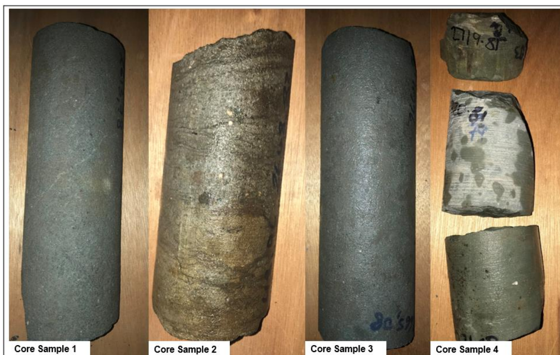
Figure 5.6 Core samples for well F-A13. Core Sample 1: 2613.78 m, Core Sample 2: 2648.82 – 2648.96 m, Core Sample 3: 2664.2 – 2665.08 m, Core Sample 4: 2719.81 m.
