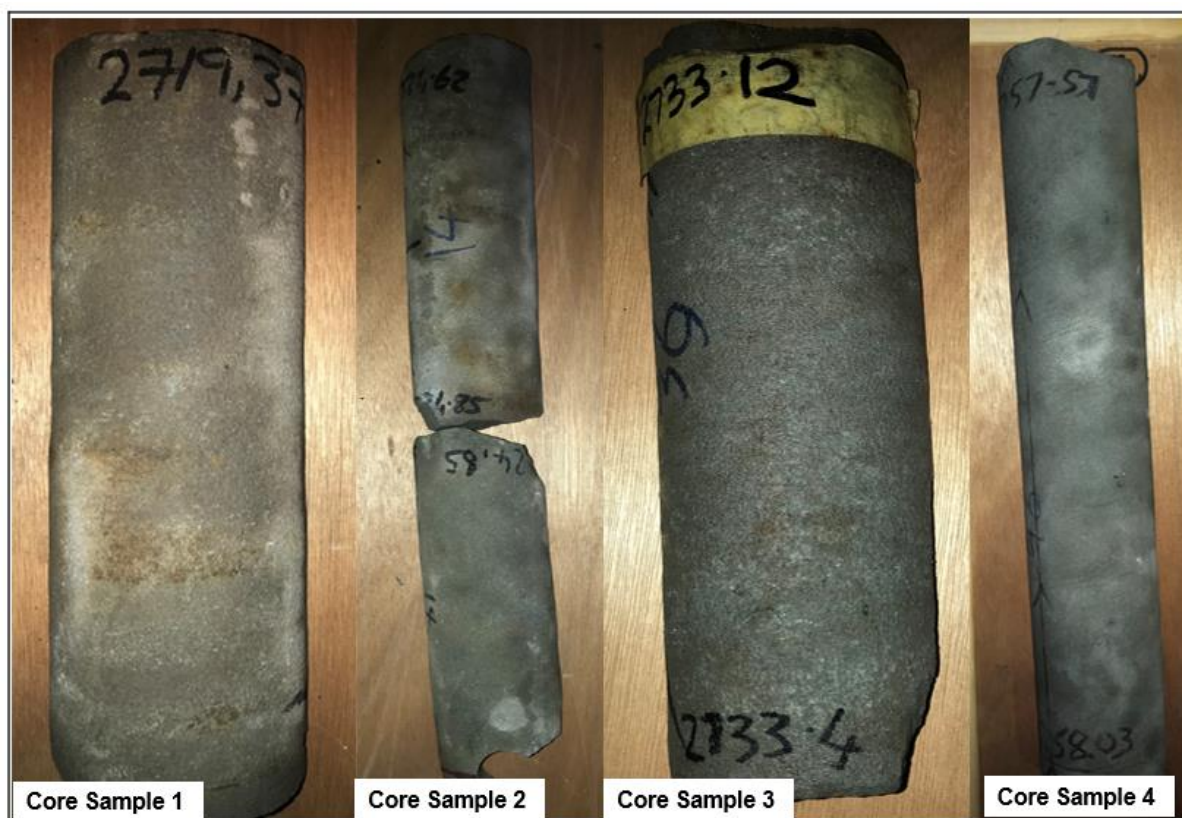
Figure 5.5 Core samples for F-A10. Core Sample 1: 2719.37 m, Core Sample 2: 2724.62 – 2724.85 m, Core Sample 3: 2733.12 – 2733.4 m, Core Sample 4: 2757.57 - 2758.03 m.
